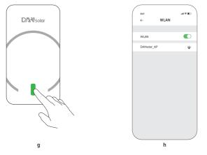
10 / Long press the LED light on the ECU unit until the light flashes red and green alternately (Picture g).
